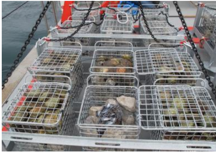
Figure 36. Oyster restoration tables installed at the scour protection of selected turbines.
