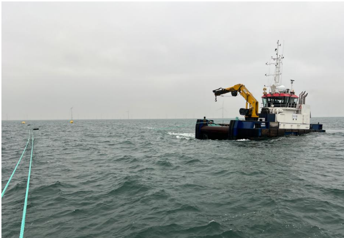
Figure 25. Dutch pilot. Multicat DP1 installing longlines (photo: OOS).
