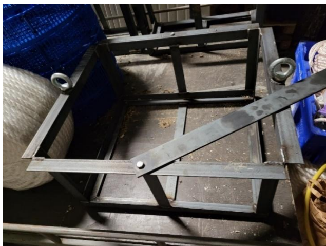
Figure 26: Frame design to add stacked SEAPA-baskets in a 2 x 2 arrangement
