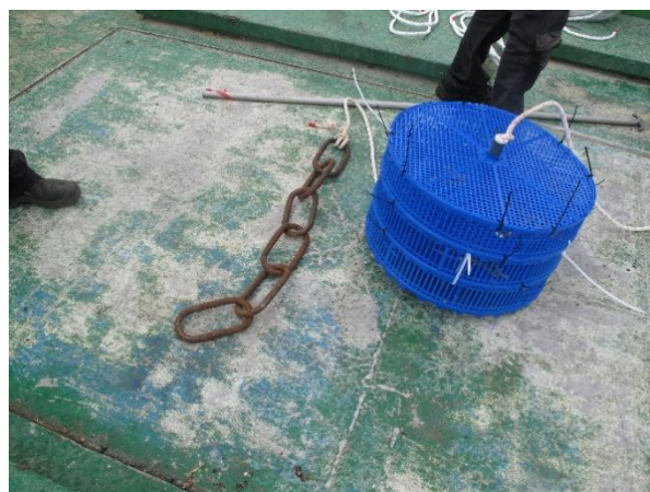
Figure 32: blue lantern baskets (Ostriga) with weights connected at the lower end of the rope
