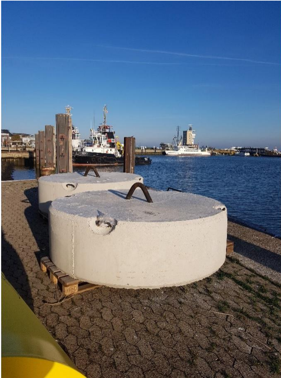
Figure 6: Six ton concrete block for mooring of the algae system
