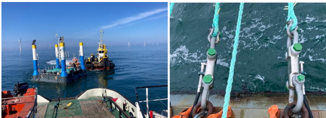
Figure 18: Test SMF being towed to location in Borssele windfarm and 2 longlines with loadcells.
